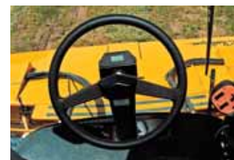
The two-spoke steering wheel provides a better view of the header and can be tilted to one of five positions for optimal operator comfort.
