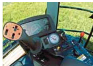
A single header/travel control lever puts all frequently used controls in the operator's right hand. In addition to speed and direction changes, the lever controls several header functions via a series of thumb switches. Depending upon the header in use, functions include header lift, swathboard actuation, draper shift and header tilt.
