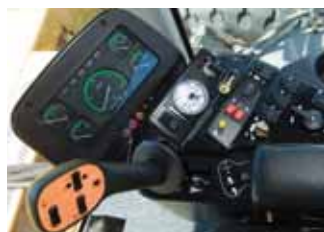
The monitor panel on the SP115B and SP185C features a row of indicator lights to warn the operator of problems, or the need to immediately stop the engine.
