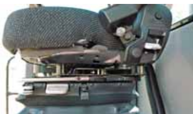
An air-suspension seat is standard equipment on "B" Series windrowers. The new seat has an adjustable headrest, adjustable backrest with adjustable lumbar support, isolator and shock absorber controls in addition to the normal fore/aft and height adjustment. The new retractable seat belt reduces the possibility of the belt getting tangled while not in use.
