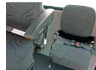
The standard instructional seat and seat belt, which now includes a backrest, folds for easy access to the cab; yet is readily available when needed by an instructor.
